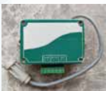
Temperature and Humidity Sensor
